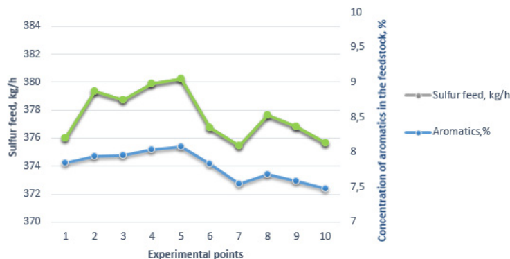
Fig. 1. Dynamics of the change in sulfur supply for combustion from the content of aromatic compounds in raw materials
